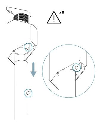
Connect the upper and lower part of the safety net poles. Make sure that all the spring clips are locked into position to keep the poles securely connected. Cover the poles with foam.
